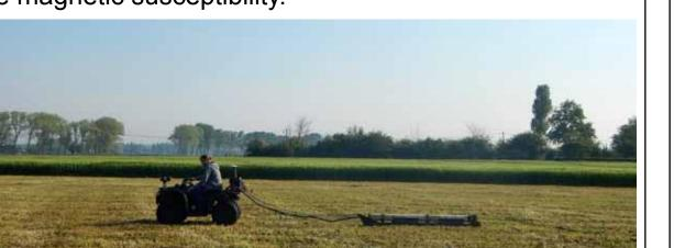
b) stepped-frequency continuous wave **GPR** operating over a frequency range from 100 to 3000MHz
