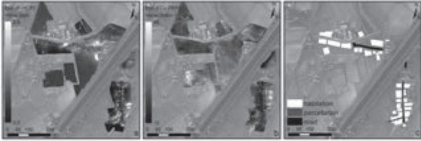
Fig. 9. Results of the geophysical survey in Monnikerede, including the magnetic response (IP) (a), the electrical conductivity (ECa) (b), and the interpretation (c). Trachet and others, ‘Reassessing Artefact Scatters’.
